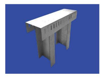
**b. Double Track (Overtrack System)** - consists of two tracks (runners). First one is called deep runner and it will be oversized (compared to the stud width by 1/8" (3mm), and it will have long flanges not less than 2" (50 mm). The deep runner is to be secured to the structure. The second track is a normal track that fits inside the deep runner.
